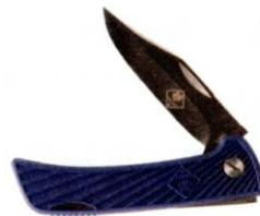
This is a jackknife. A jackknife is a good tool for campers and fishermen. It has a hinged blade at only one end and may have one or two blades. Some jackknives (and other knives) have locking blades. That means you have to push a release before you can close the blade. Locking blades prevent you from accidentally closing the blade on your fingers.
